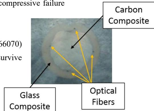
short exposure times to high temperatures during pultrusion and monitor relatively low-magnitude bending and axial tension strains in a composite material. The optimal placement of embedded optical fibers in the rods was determined based on the rods' limitations and the mechanical strength of the commercially available optical fibers.
