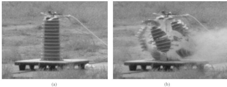
In this unique study, conducted jointly by the HVT Center, the US Bureau of Reclamation, and the FBI, HV porcelain transformer bushings subjected to high-power rifle damage were experimentally modeled as
